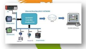
Solution for Industrial Network Ethernet, MODBUS, IOT & Remote communication.
